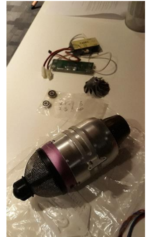
A modern model turbine, ceramic bearings, Garrett impeller and electronic bits.
